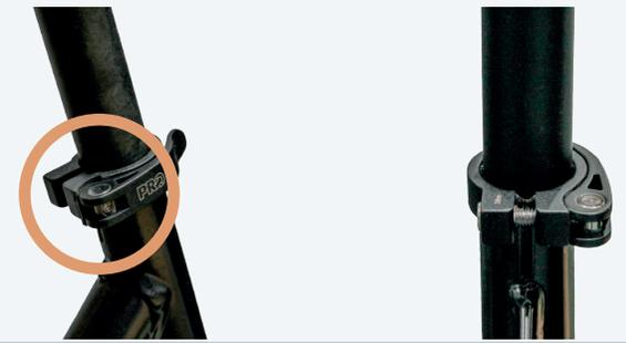
**Please Note:** When tightened, there is approximately 2 mm distance between the quick release handle and the locking mechanism's outer surface (see the figure to the right).
