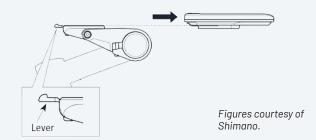
Push the lever downwards and slide the cycle display outwards.
