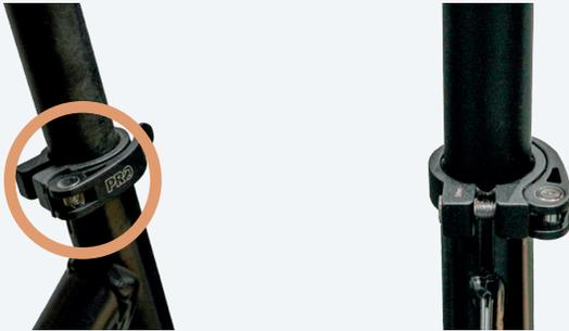
**Please Note:** That, when tightened, there is approximately 2 mm distance between the quick release handle and the locking mechanism’s outer surface (see the figure to the right).
