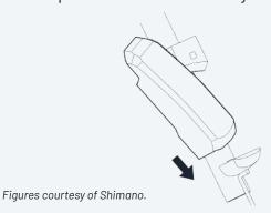
Removing the battery from the battery mount:
